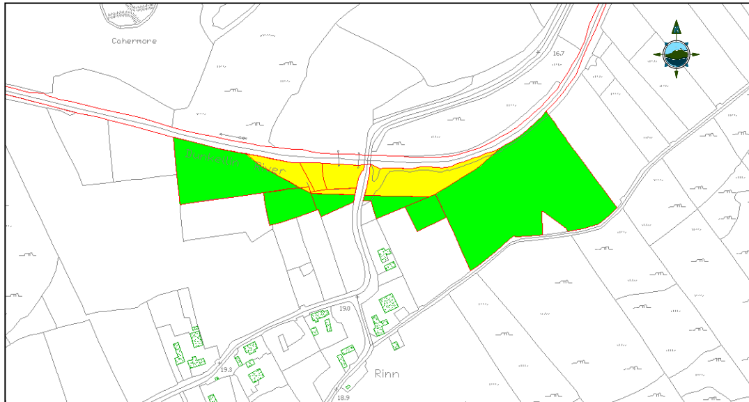
Figure 6-4 – Approximate Location of Lands required for deposition of excavated material (green) upstream of Rinn Bridge (Yellow Areas indicate extent of channel excavations)
